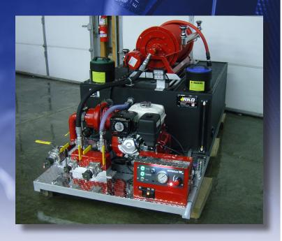
This slip on end mount firefighting unit is designed by us to fit a standard 8 foot or 6.5 foot truck bed.
